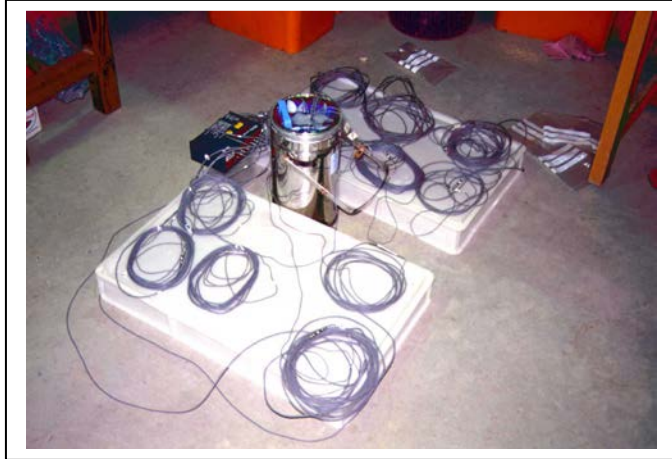
Fig. 19 Squirrel data logger probes being calibrated in an ice/water slurry prior to treatment commencement.
