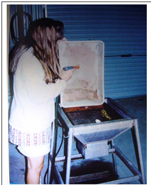
Fig. 15 For Basic (Most tolerant Stage) tests infested Test and Control grapes were placed in these trays at 1°C (Test fruit) or 26°C (Control fruit).
