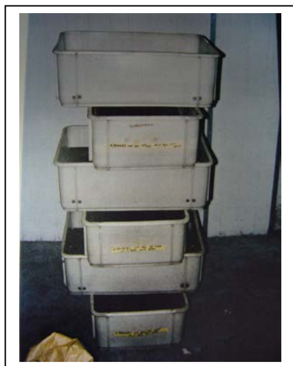
Fig. 15 For Basic (Most tolerant Stage) tests infested Test and Control grapes were placed in these trays at 1°C (Test fruit) or 26°C (Control fruit).
