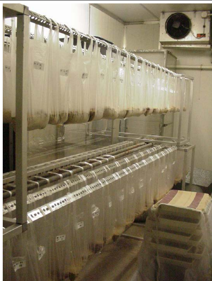
Fig. 32 Infested grapes are placed into plastic bags with damp vermiculite (pupation medium) at either 2°C or 3°C for determination of the most cold-tolerant life stage.
