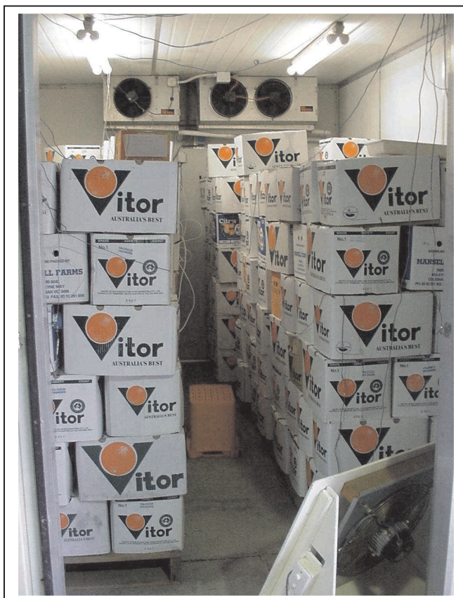
Figure 12 Filler fruit, apples in citrus cartons surround summerfruit cartons with infested summerfruit and non-infested summerfruit that are monitored for temperature (the temperature probe cables connecting the summerfruit to the data logger can be seen suspended from the ceiling).
