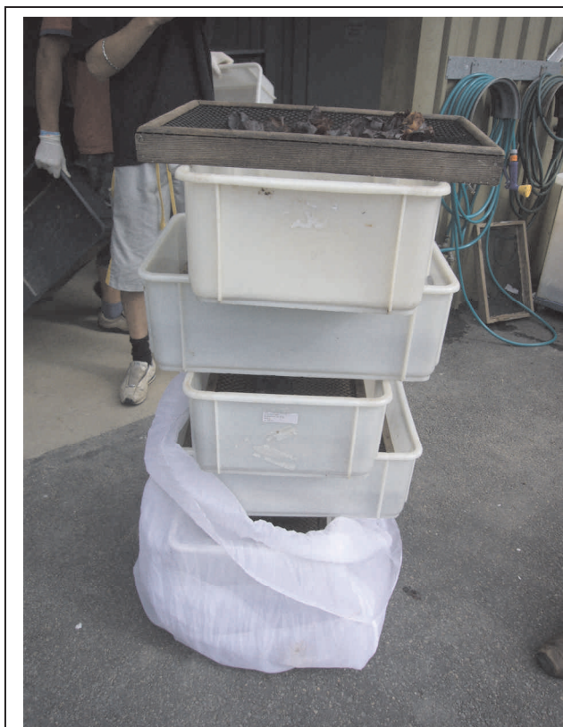
Figure 26 The mesh trays with infested fruit on top are placed inside a large plastic tub which are stacked allowing adequate ventilation. The stack is then covered with a fine terylene netting to stop contamination by Drosophila spp. (vinegar flies).
